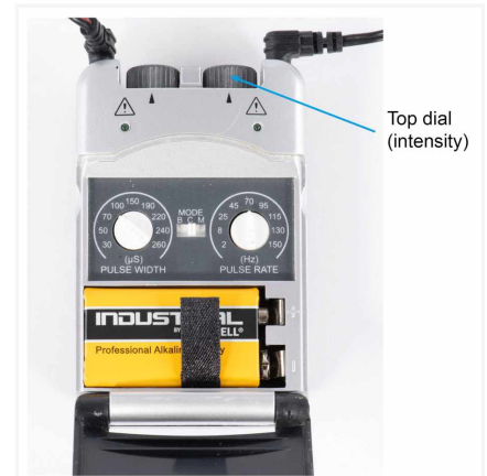
3. Switch on the machine and turn up the intensity (top dial) until you feel a comfortable tingle.
