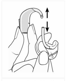
Step 1: Remove the old existing tubing with your hand or pliers. Please keep the removed tubing to use for sizing later on.
