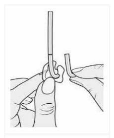
Step 2: Use the removed tubing from step 1 as a guide to cut the new tubing to your exact and preferred length. Carefully cut it at the same length.
